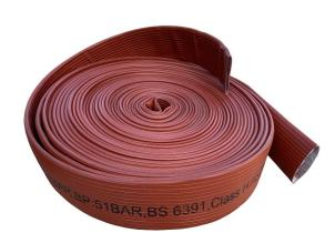
Fortex is an extruded rubber hose for professional firefighting applications. It is made by weaving high-tenacity yarns and covering the textile reinforcement with a synthetic rubber compound. This process creates a high-pressure fire hose that is abrasion and chemical resistant.
