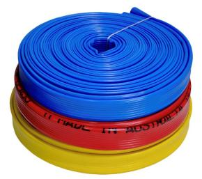
**Rapier** has had an upgrade. Woven with state-of-the-art Loomex<sup>™</sup> technology, **Rapier** has a fused thermoplastic polyurethane lining, creating an inseparable bond with the textile reinforcement. This Type 3 fire hose is extruded with a PVC/Nitrile rubber blend cover, which protects it against abrasion damage and makes it easy to wipe clean of oils, stains, and dirt. It is a popular choice for both fire brigades and industrial plant protection.
