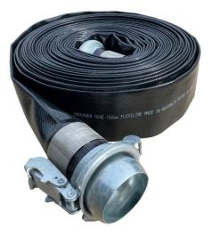
**Flexiline** is a flexible layflat hose used for industrial pumping applications. It is robust and typically used for pumping pressures operating up to 1500 kPa. It can be supplied with a large range of couplings, including Bauer for quick-connect dewatering use.
