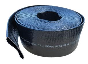
Flexiline is a flexible layflat hose used for industrial pumping applications. It is robust and typically used for pumping pressures operating up to 1500 kPa. It can be supplied with a large range of couplings, including Bauer, for quick-connect dewatering use.
